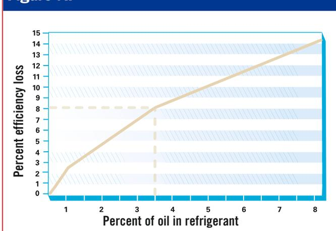
The graph shows the impact of oil content in refrigerant in terms of efficiency loss.
